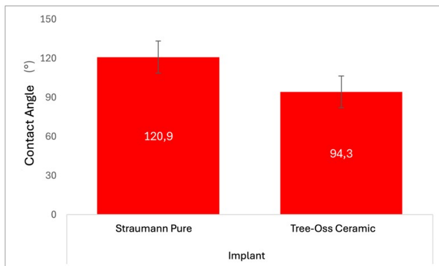
Figure 4: Mean and standard deviation obtained for the contact angle of the implant surface measured by Goniometer.
