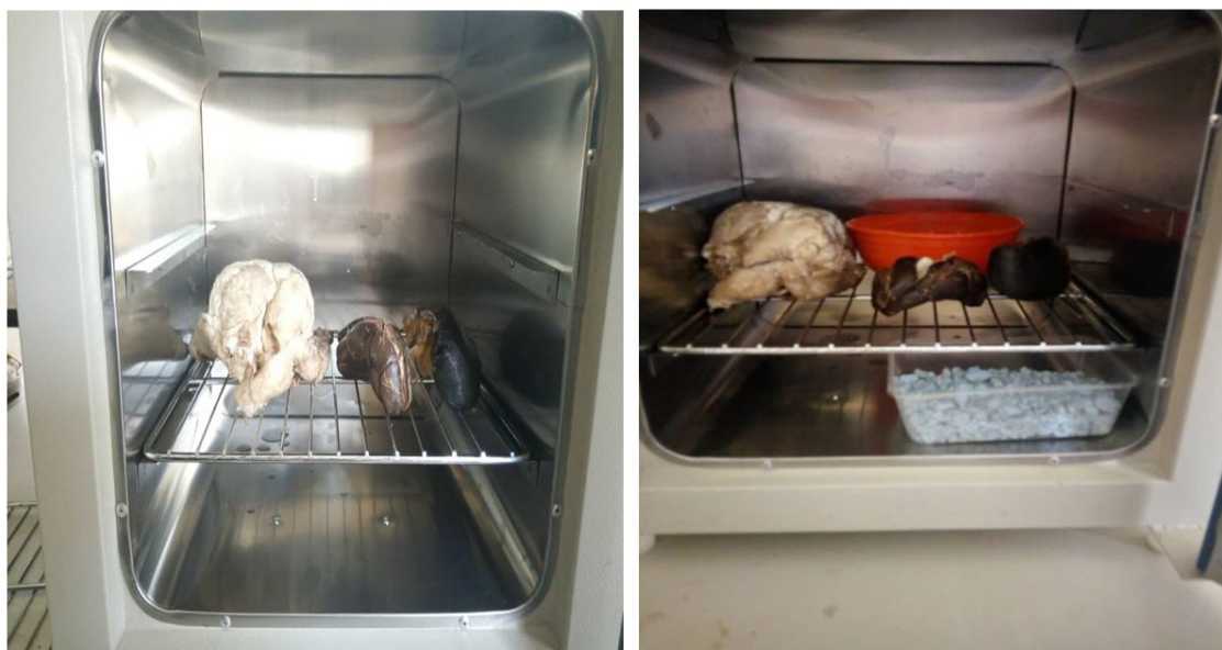
Figure 3: Showing an improvised curing stage using an oven as a curing chamber with specimen neatly arranged. It also contains BIODUR S6 as the curing gas and potassium acetate for dehydrating
