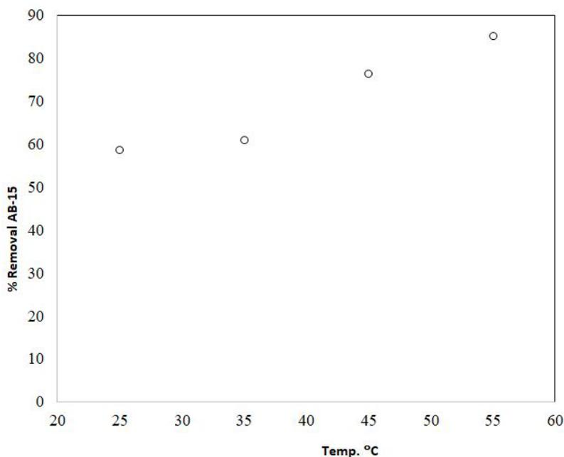
Figure 2: Effect of temperature (dosage of Fe (III)-chitosan sorbent = 2 g L<sup>-1</sup>, C<sub>i</sub> = 100 mg L<sup>-1</sup>, 80 rpm, pH<sub>i</sub> = 7.00)
