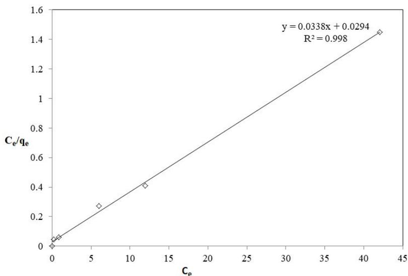
**Figure 5:** The linearized Langmuir adsorption isotherms for AB-15 adsorption onto Fe (III)-chitosan complex sorbent (dosage = 2 g L<sup>-1</sup>, Temperature = 35 °C, agitation speed = 80 rpm and contact time = 50 min)
