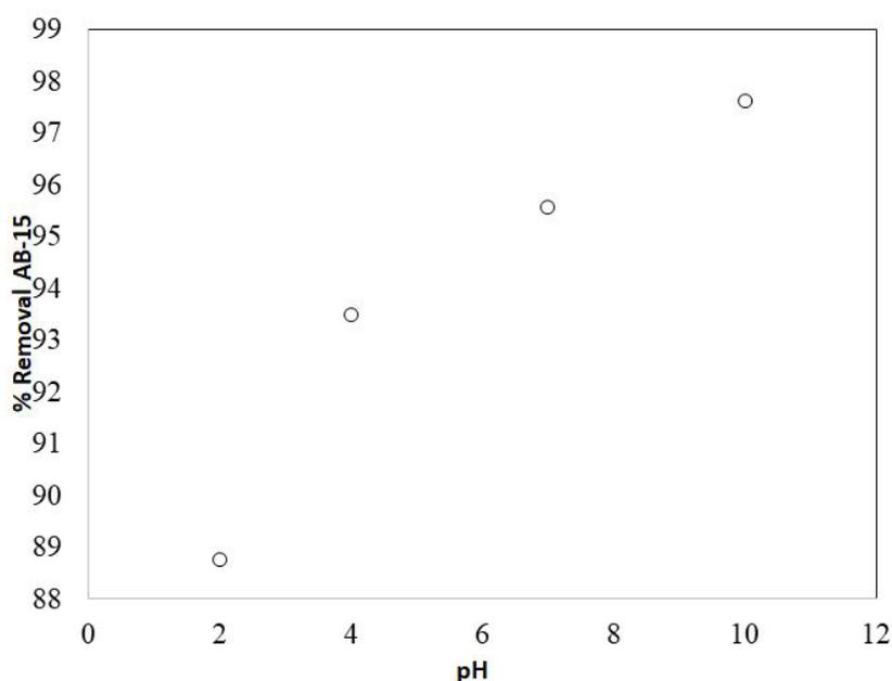
Figure 4: Effect of pH (t = 90 min, C<sub>i</sub> = 100 mg L<sup>-1</sup>, 35 °C, dosage of Fe (III)-chitosan complex = 2 g L<sup>-1</sup>, 80 rpm)
