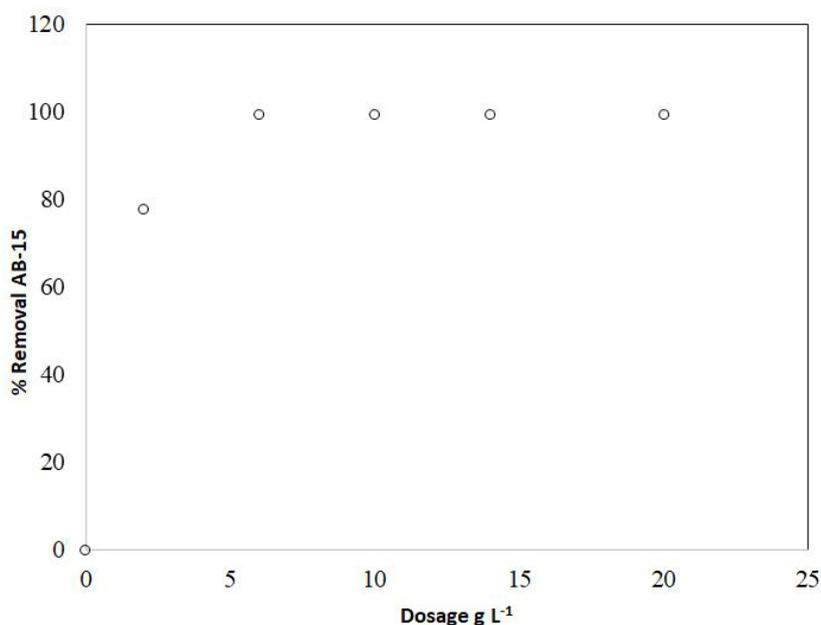
Figure 3: Effect of Fe (III)-chitosan complex sorbent dosage (t = 50 min, 50 ml, T = 35 °C, C<sub>i</sub> = 100 mg L<sup>-1</sup>, 80 rpm, pH<sub>i</sub> = 7.00)
