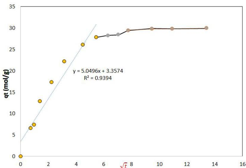
Figure 11: Weber-Moris intra-particle diffusion kinetic model,  $T = 55\text{ }^{\circ}\text{C}$ ,  $t = 30\text{ min}$ ,  $C_i = 100\text{ mg L}^{-1}$
