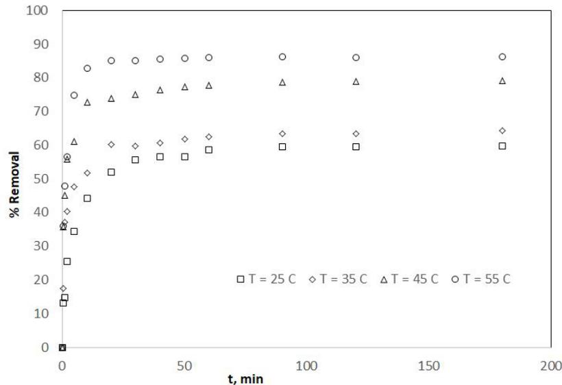
**Figure 8:** Effect of contact time on AB-15 sorption by using different temperature (25, 35, 45, and 55 °C), dosage = 2 g L<sup>-1</sup>, 80 rpm, and C<sub>i</sub> = 100 mg L<sup>-1</sup>, pH<sub>i</sub> = 7.0
