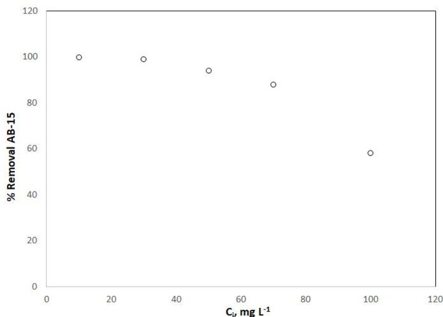
**Figure 1:** Effect of initial concentration of AB-15 ( $t = 50$  min,  $35\text{ }^\circ\text{C}$ ,  $50\text{ ml}$ ,  $0.1\text{ g}$  Fe (III)-chitosan complex sorbent,  $80\text{ rpm}$ )
