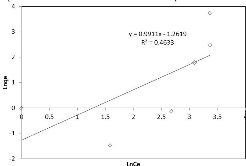
**Figure 6:** The linearized Freundlich adsorption isotherms for AB-15 adsorption by Fe (III)-chitosan complex sorbent (dosage = 2 g L<sup>-1</sup>, Temperature = 35 °C, agitation speed = 80 rpm and contact time = 50 min)
