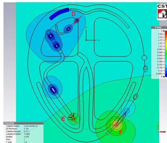
Figure 5: 2D view of the potential field spread in biventricular stimulation and intersection at the level of the right ventricular electrode
