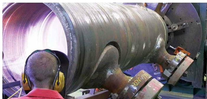
Figure 6: Weld hardfacing of a cylinder for corrosion resistant https://www.arcenergy.co.uk )
