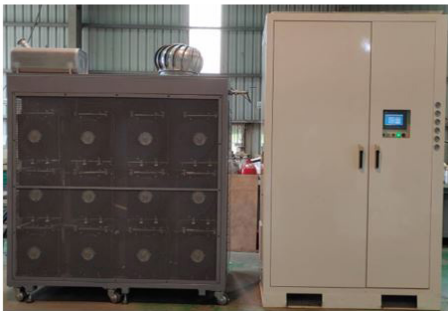
Figure 1: A 30Nm 3 /h hydrogen generator (R) and a 30kW fuel cell stack (L)
