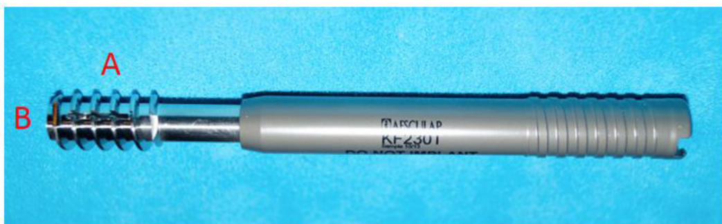
Figure 1: For augmentation with CPC, standard telescopic screws of the Targon System have been perforated by the manufacturer (Aesculap AG) over the full length, with two additional fenestrations at the head of the screw (A); The tip of the screw (B) was closed
