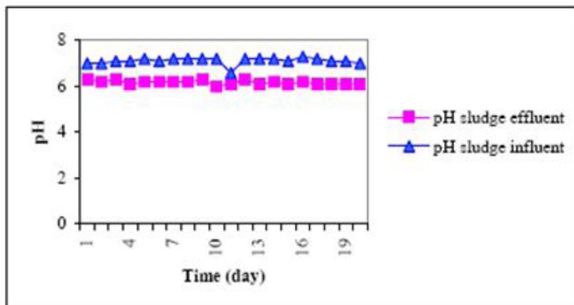
Figure 6: Potential of hydrogen sludge before and after treatment in the digester [12]
