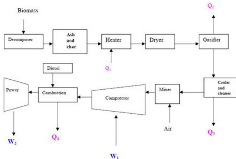
Figure 7: Advanced biomass power with diesel engine [12]
