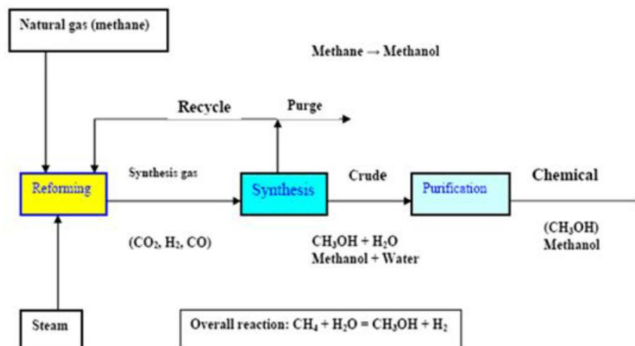
Figure 2: Schematic diagram shows methanol production [12]
