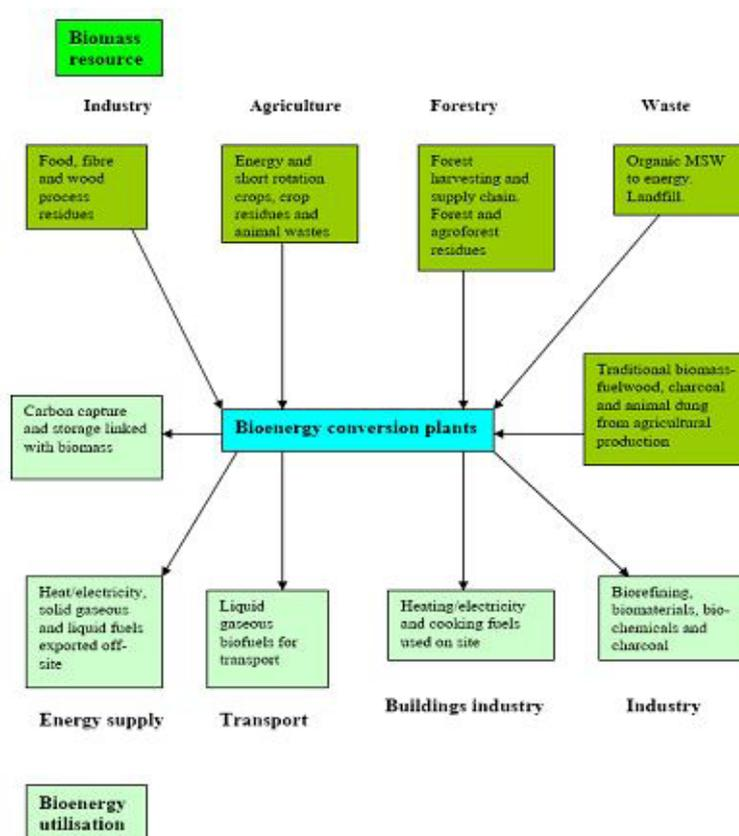
Figure 4: Biomass resources from several sources are converted into a range of products for use by transport, industry and building sectors [21]
