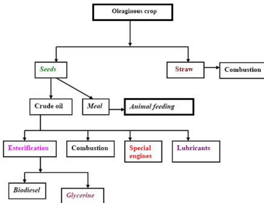
Figure 9: Flow chart of biodiesel production [12]
