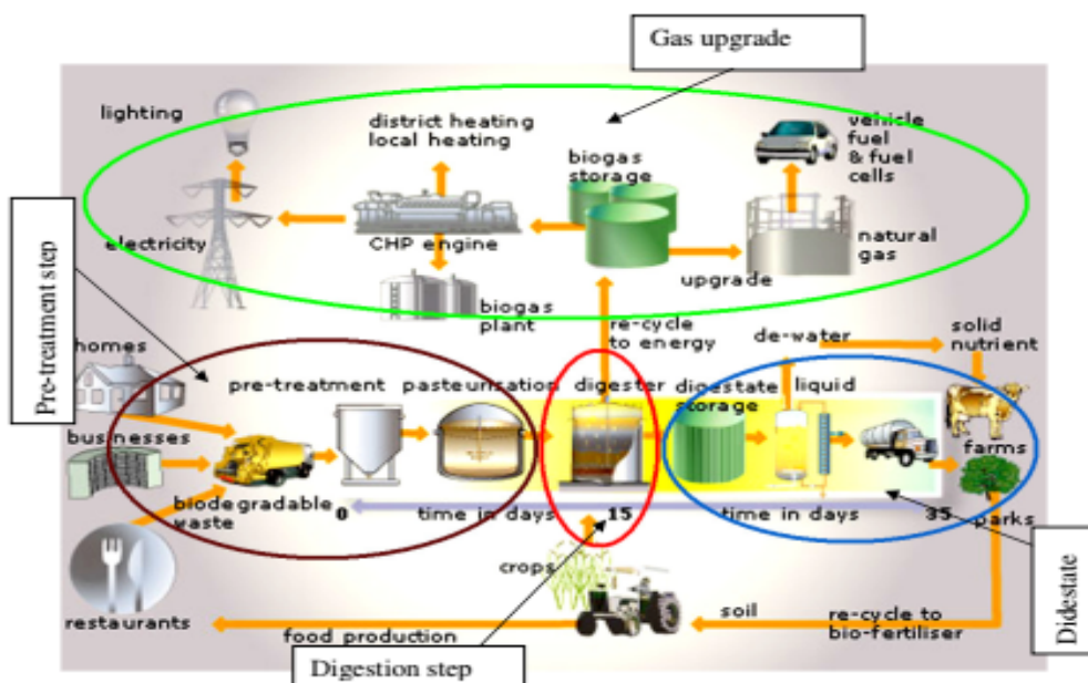
Figure 1: Diagram of general process of AD in electricity production through biomass by combustion
