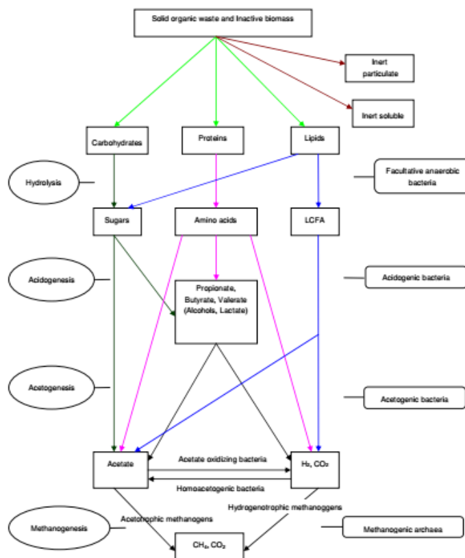
Figure 4: Main steps and pathways of dry anaerobic digestion process
